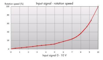
The input signal is directly proportional to the efficiency of the wheel, which means that input signal and rotation speed are as per adjoining diagram.
